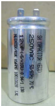
Running Capacitor 250VAC-12 \mu F
