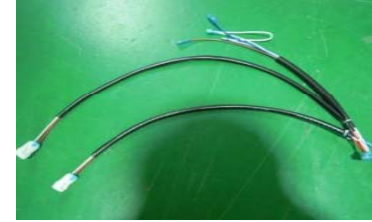
HARNESS COMP Compressor Type [[SK1A1C-L1U2]
